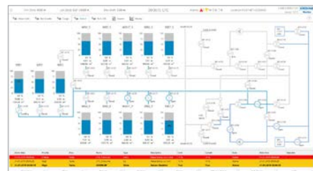
Ballast tank view
